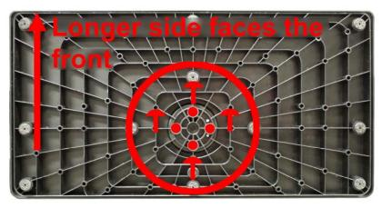
2. To remove the stand, remove the 5 screws in the circled area and the stand will come off.
