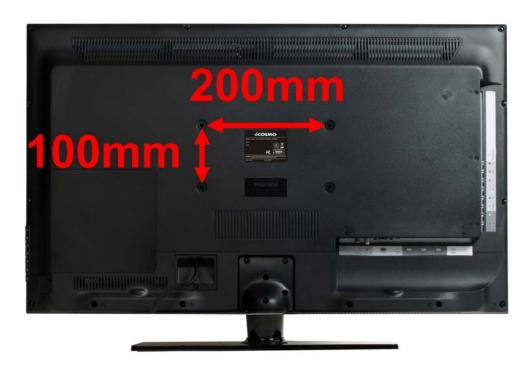
Mounting Specification: **200mm x 100mm** using screw size **M6**. Length of screw should not exceed **18mm**. Please Note: The 18**mm** length of screw refers to how deep the screw can go inside the mounting holes. When you're buying screws, you should add the original 18mm to the thickness of your mounting plate in order to get the total screw length.
