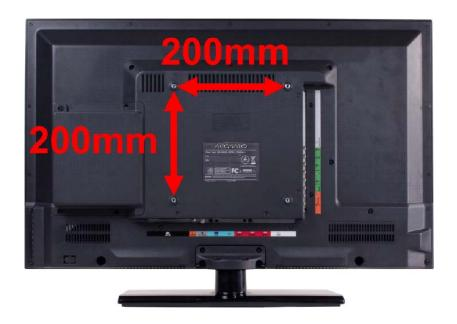
Mounting Specification: **200mm x 200mm** using screw size **M5**. Length of screw should not exceed **9mm**. Please Note: The **9mm** length of screw refers to how deep the screw can go inside the mounting holes. When you're buying screws, you should add the original 8mm to the thickness of your mounting plate in order to get the total screw length.
