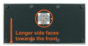
2. To remove the stand, remove the 4 screws indicated in the picture and the stand will come off.
