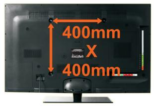
Mounting Specification: **400mm x 400mm** using screw size **M6**. Length of screw should not exceed **30mm**. Please Note: The **30mm** length of screw refers to how deep the screw can go inside the mounting holes. When you're buying screws, you should add the original 30mm to the thickness of your mounting plate in order to get the total screw length.
